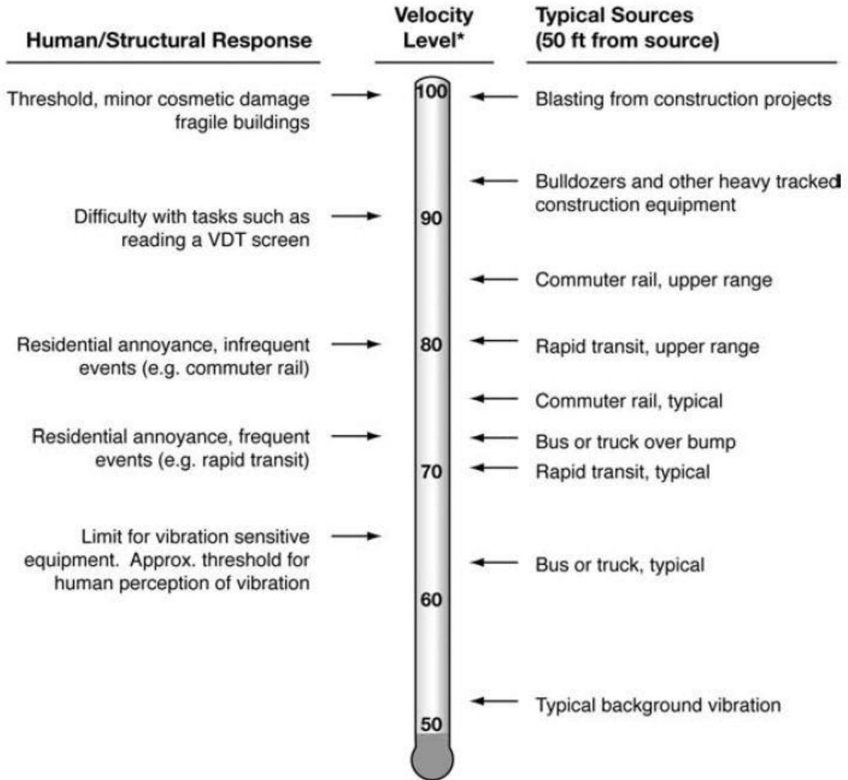
\* RMS Vibration Velocity Level in VdB relative to  $10^{-6}$  inches/second
