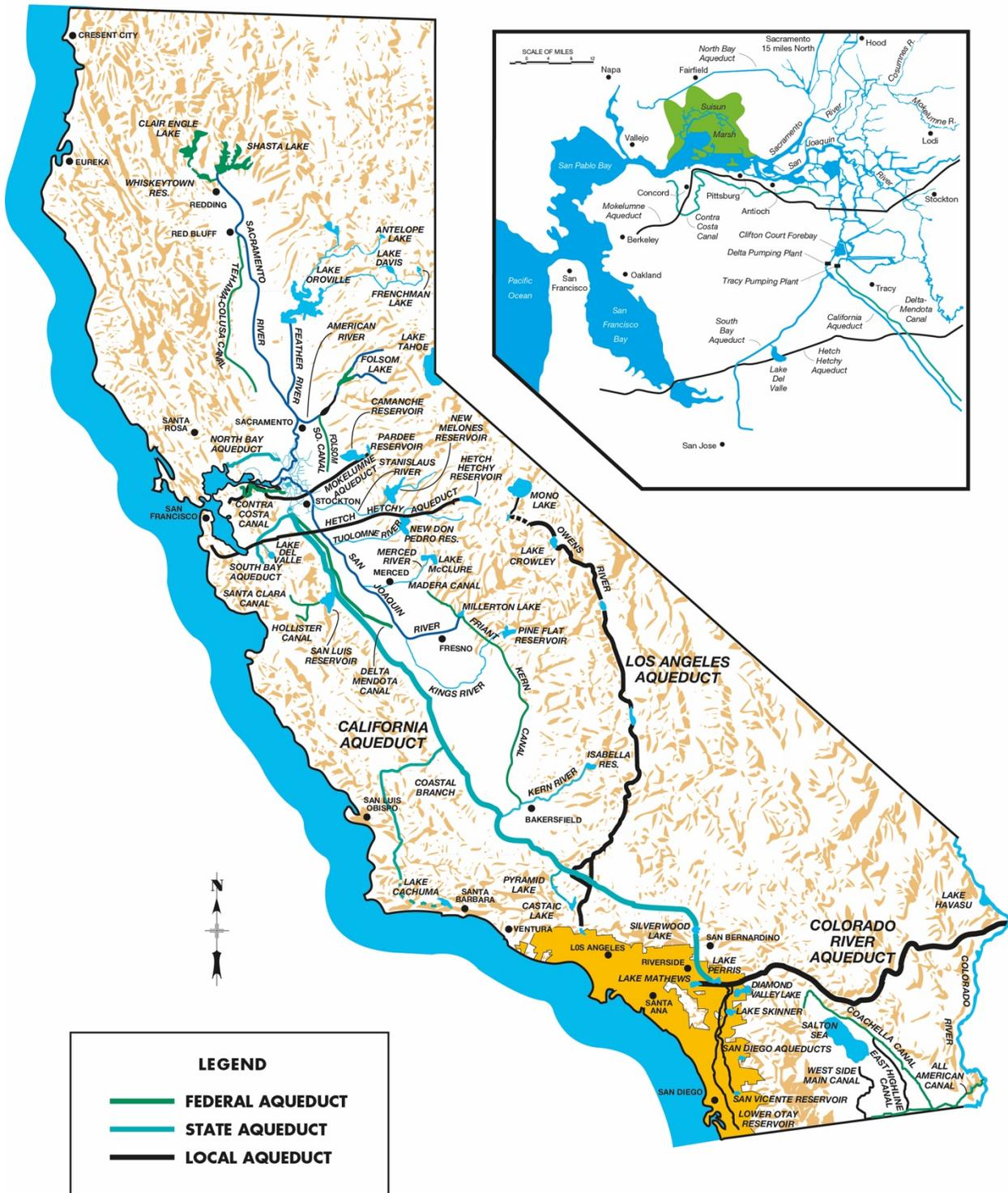
The water is delivered to Metropolitan's service area by way of the CRA, which has a rated capacity of approximately 1,700 cfs. The CRA conveys water 242 miles from its Lake Havasu intake to its terminal reservoir, Lake Mathews, near the City of Riverside. Conveyance losses along the CRA of 10 TAF per year reduce the amount of Colorado River water received in the coastal plain.
