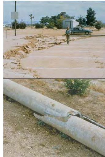
The photograph on the left shows a pipe joint pullout due to liquefaction from 1995 in Kobe, Japan. (photo courtesy of D. Ballantyne, *Understanding the Seismic Vulnerability of Water Systems*, Regional Water Providers Consortium Board, October 2013)
